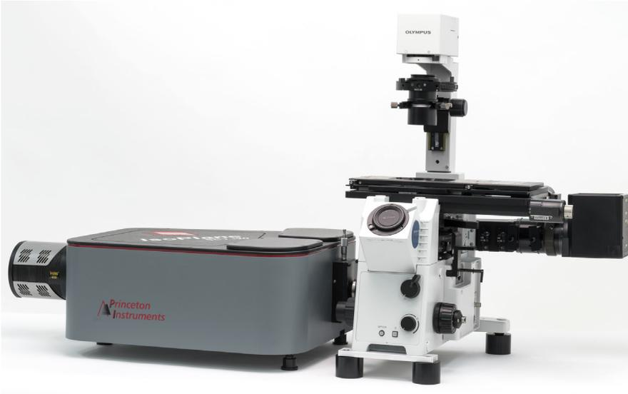
IsoPlane spectrograph shown interfaced to Olympus IX-71 inverted microscope with the IsoPlane microspectroscopy interface (spectrograph, microscope, camera, and interface all sold separately). Contact your local sales engineer for more information.
